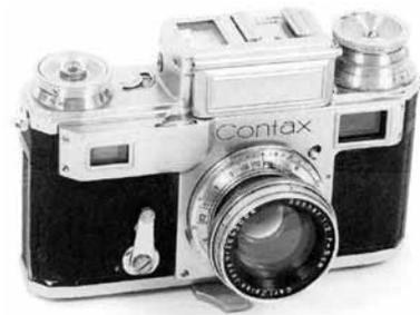
years. Then, you set your camera controls by consulting instructions that came with the film: full sun, partly cloudy, shade, snow, etcetera, and hoped for the best. The Contax had a built-in light meter that eliminated guess work, as well as a range finder for focusing, a delayed-action shutter release, and a lens the size of a golf ball for dark scenes. There was nothing like it.
